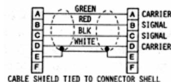
To minimize pickup from nearby AC power sources or lines, always use shielded cable. Also, it is best not to run transducer cables in trays or conduits carrying AC power. Because the 3 or 5 kHz transducer signal is about 200 mV rms full scale, a high current 230 Vac line lying next to it can cause an excessive 60 Hz noise signal.
