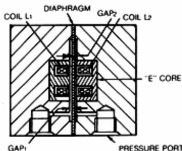
FIGURE 1. Typical Transducer Cross-Section
